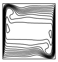
Fig. 2. Isolines of temperature (left) and stream function (right) for flow ina square cavity with side heating for H/L=1, Pr=0.71,  $Ra=10^7$ .
