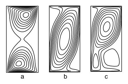
Fig. 1. A fluid flow structure (stream function) in a cavity  $\rm H/L=2$  with top and bottom moving lids for Reynolds number Re=100 (a) and symmetrical (b) and non-symmetrical (c) flows for Re=3000.
