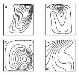
Fig. 4. Isolines of stream function for cases A3 (a), B2 (b), C2 (c) and temperature for case C2 (d) of [20].
