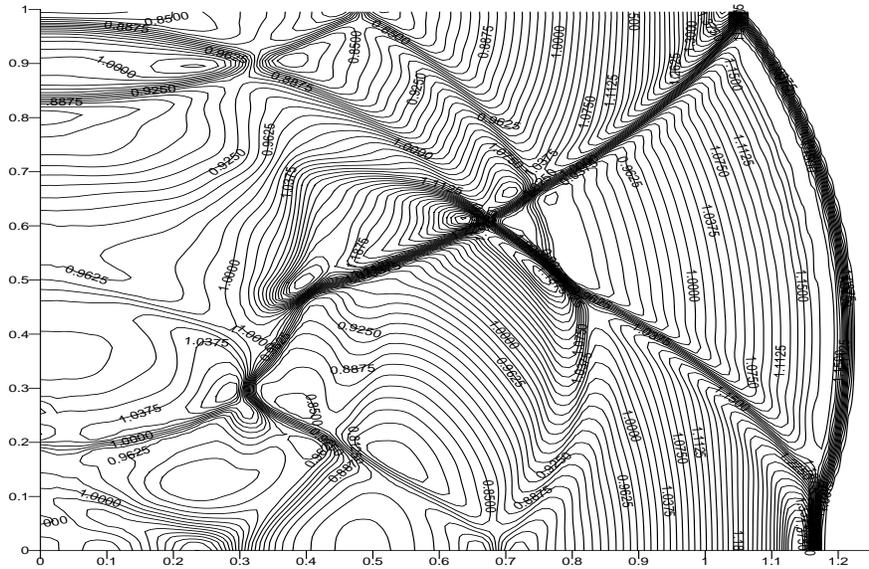
Figure 1: Pressure contours from 0.775 to 1.5 with increment 0.0125 in the  $x-z$  plane at  $t=0.7$  computed on the rectangular mesh  $100 \times 140$ .
