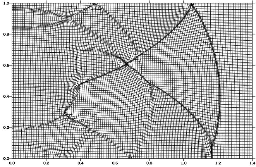
Figure 3: Adapted mesh  $100 \times 140$ ,  $p$  is a control function,  $c_\alpha=0.21$ .
