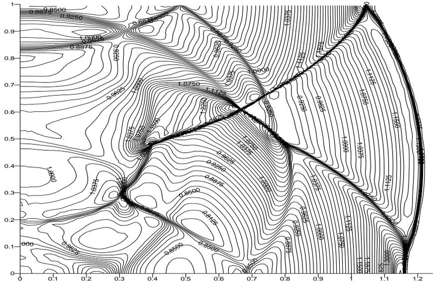
Figure 2: Pressure contours computed on the adapted mesh  $100 \times 140$ .
