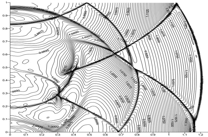
Figure 6: Pressure contours computed on the adapted mesh  $200 \times 250$ .
