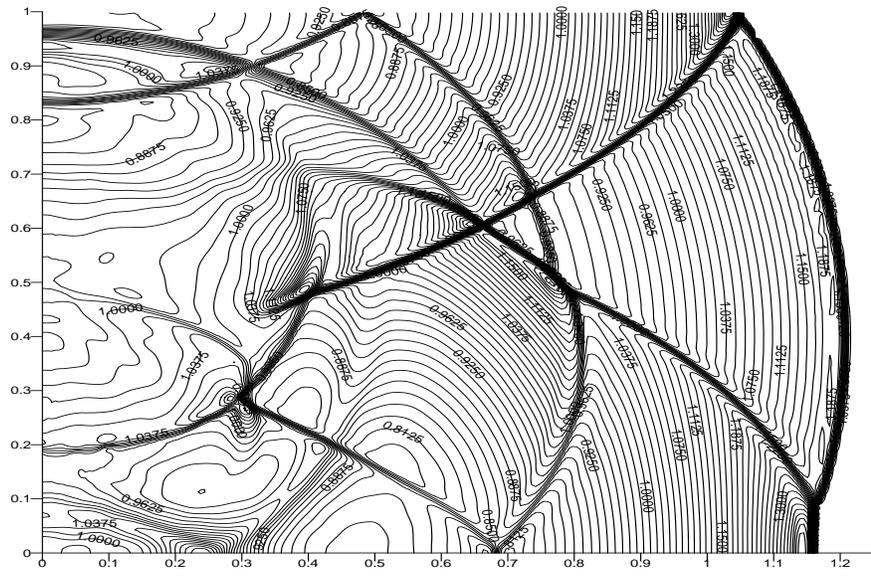
Figure 5: Pressure contours computed on the rectangular mesh  $200 \times 250$ .
