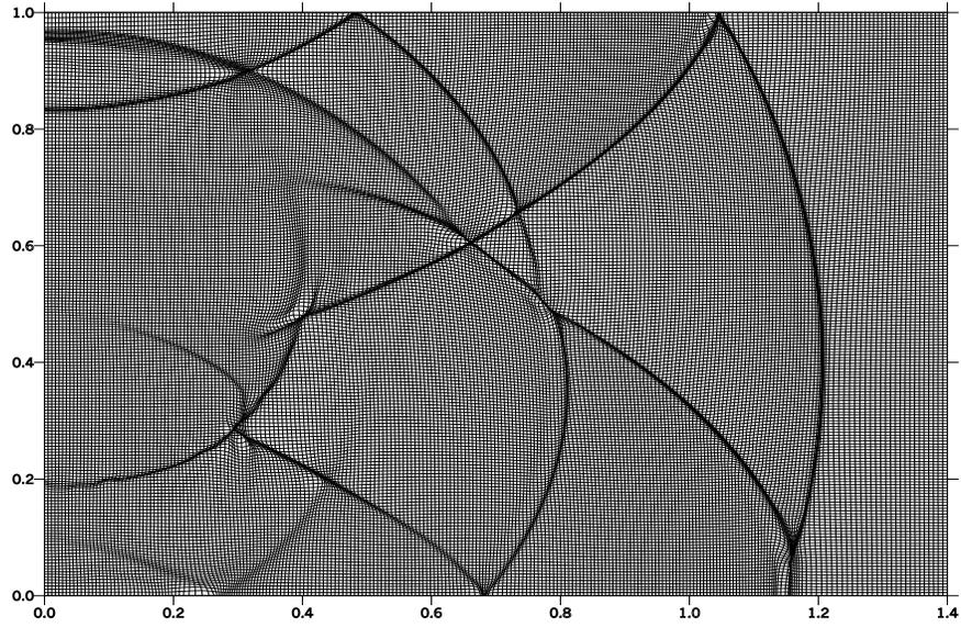
Figure 4: Adapted mesh  $200 \times 250$ ,  $p$  is a control function,  $c_\alpha=0.18$ .
