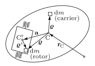
A gyrostat is a mechanical system consisting of several bodies which possesses the rigid body property, which means that the mass distribution of the system does not change over time.
