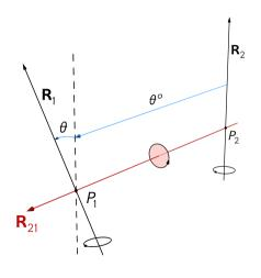
The dual angle  $\Theta = \theta + \theta^{\circ} \varepsilon$  between two axes  $\mathbf{A}_1$  and  $\mathbf{A}_2$  is a shape formed by these axes and a straight line segment  $P_2P_1$  intersecting the axes at right angles.
