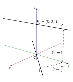
Consider the screw motion of a line l with a guide vector  $\mathbf{v} = \frac{1}{\sqrt{2}} (1, 1, 0)^T$  and passing through the origin.
