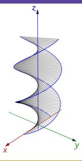
The helicoid in the figure on the left is obtained by a uniform screw motion of a straight line Ox along the Oz axis. Calculations were performed using biquaternions.
